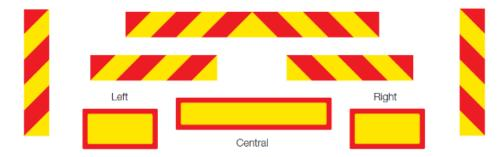
Such marking must be fully reflective vehicle signs, conforming to B.S. AU152.
