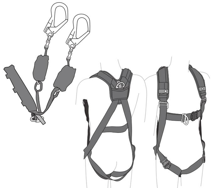
Figure 39: High specification personal fall protection equipment.
