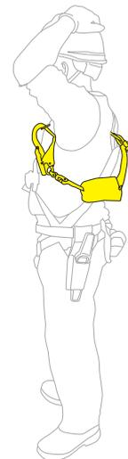
(iii). A hybrid self-retracting lanyard with minimum trailing lanyard when stowed.
