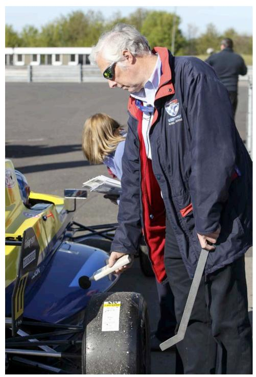
Figure 9 Official checking vehicle noise level
