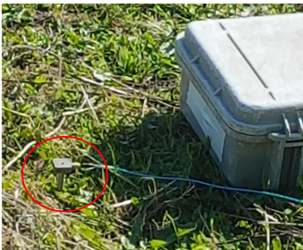
Figures C2, close-up photograph of vibration transducer and mounting position.
