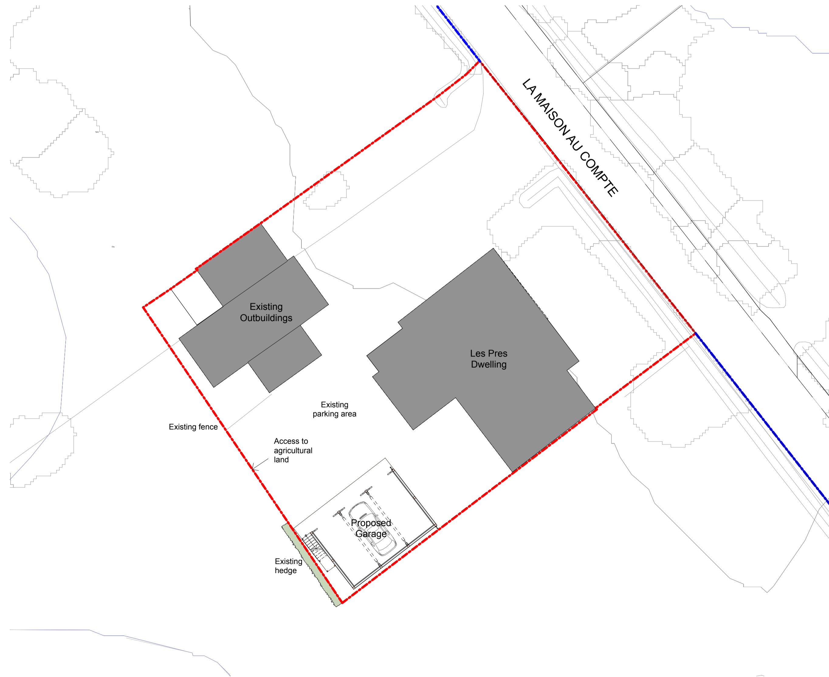
Site Layout Plan as Proposed Scale 1:200
