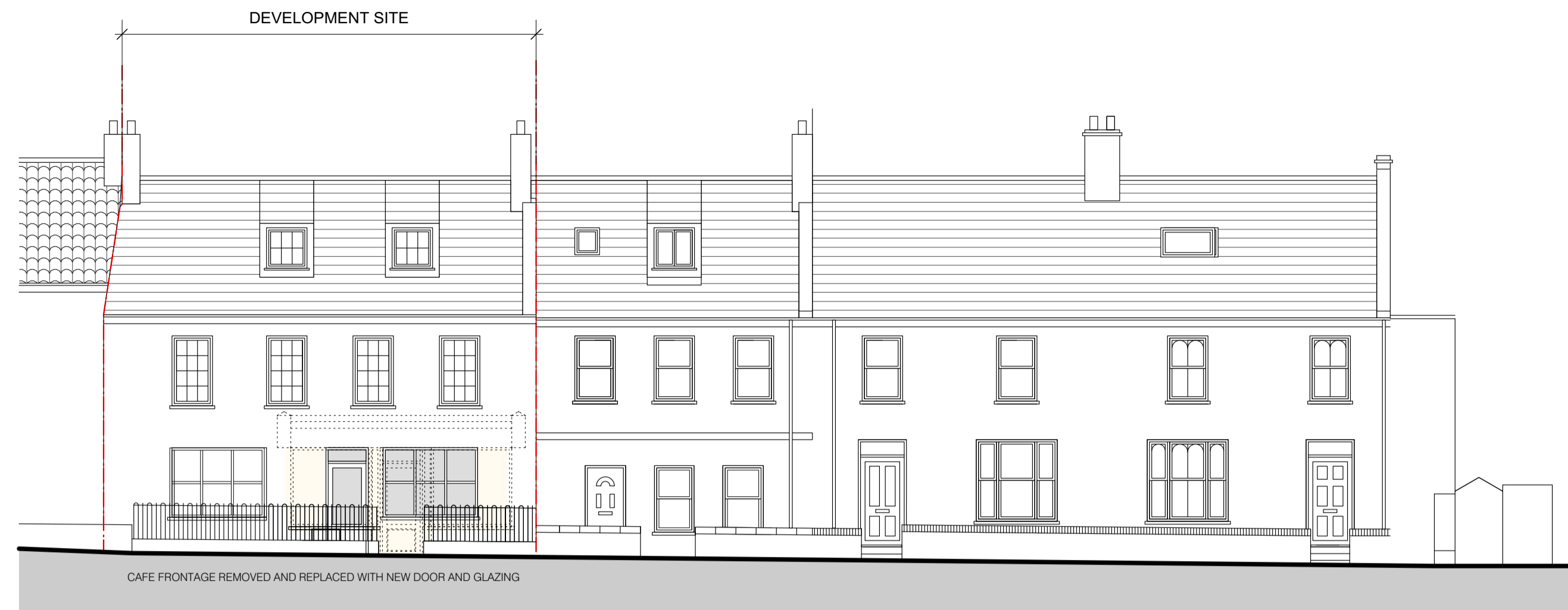
EAST ELEVATION (FLATS) SCALE: 1:100
