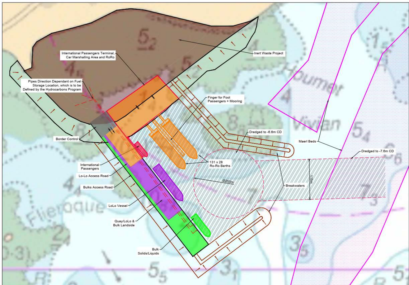
Figure 1: Layout for the new port facility – Option 3.1
