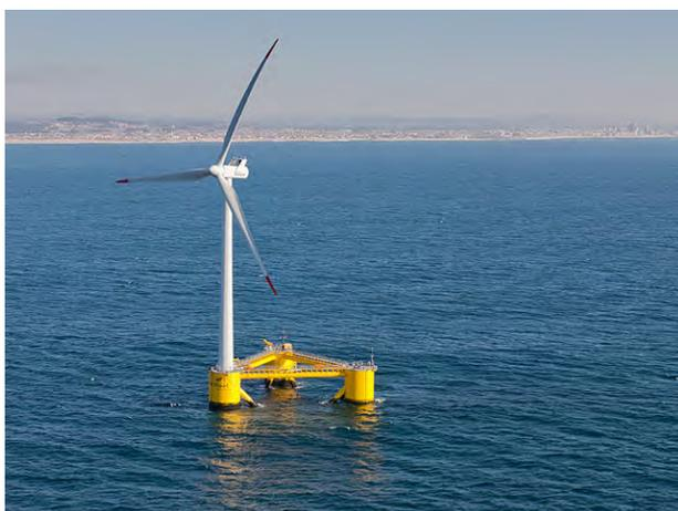
Figure 2.5 Example of Floating Wind Turbine - Windfloat by Principle Power
