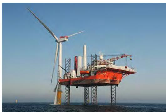
Figure 2.6 Example Construction Vessel (Jackup Barge)
