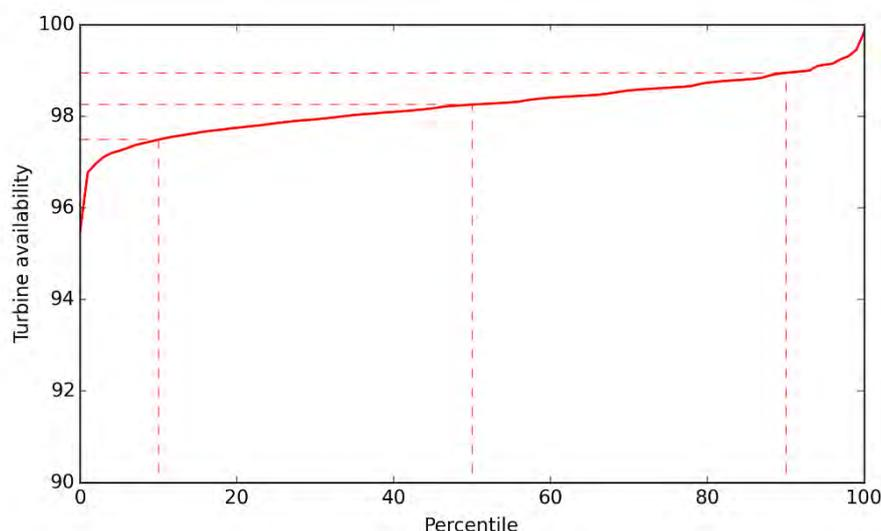
**Figure 3 – The distribution of turbine availability for 5000 Monte Carlo simulations of randomly timed major failures – for the standard simulation for fixed foundation turbines (repaired using a jack-up).**
