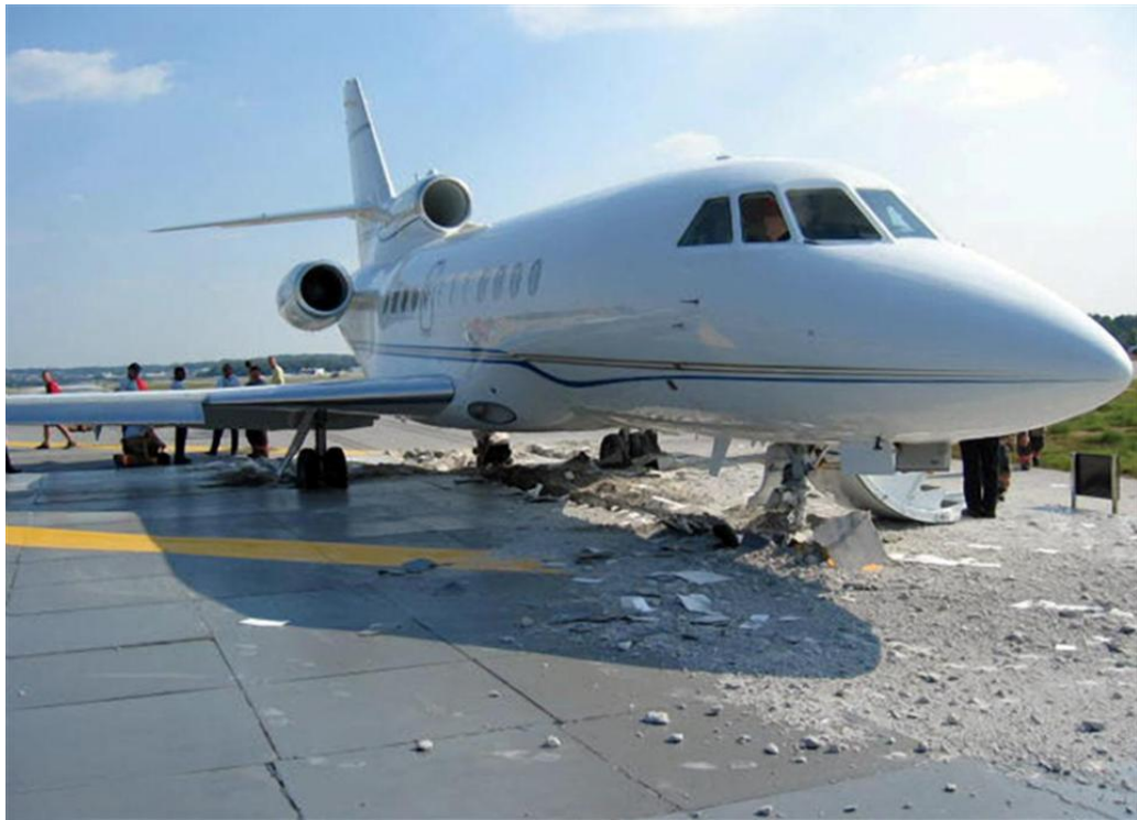
In stopping an aircraft, the aerated concrete blocks are crushed and hence following an incident blocks have to be replaced.
