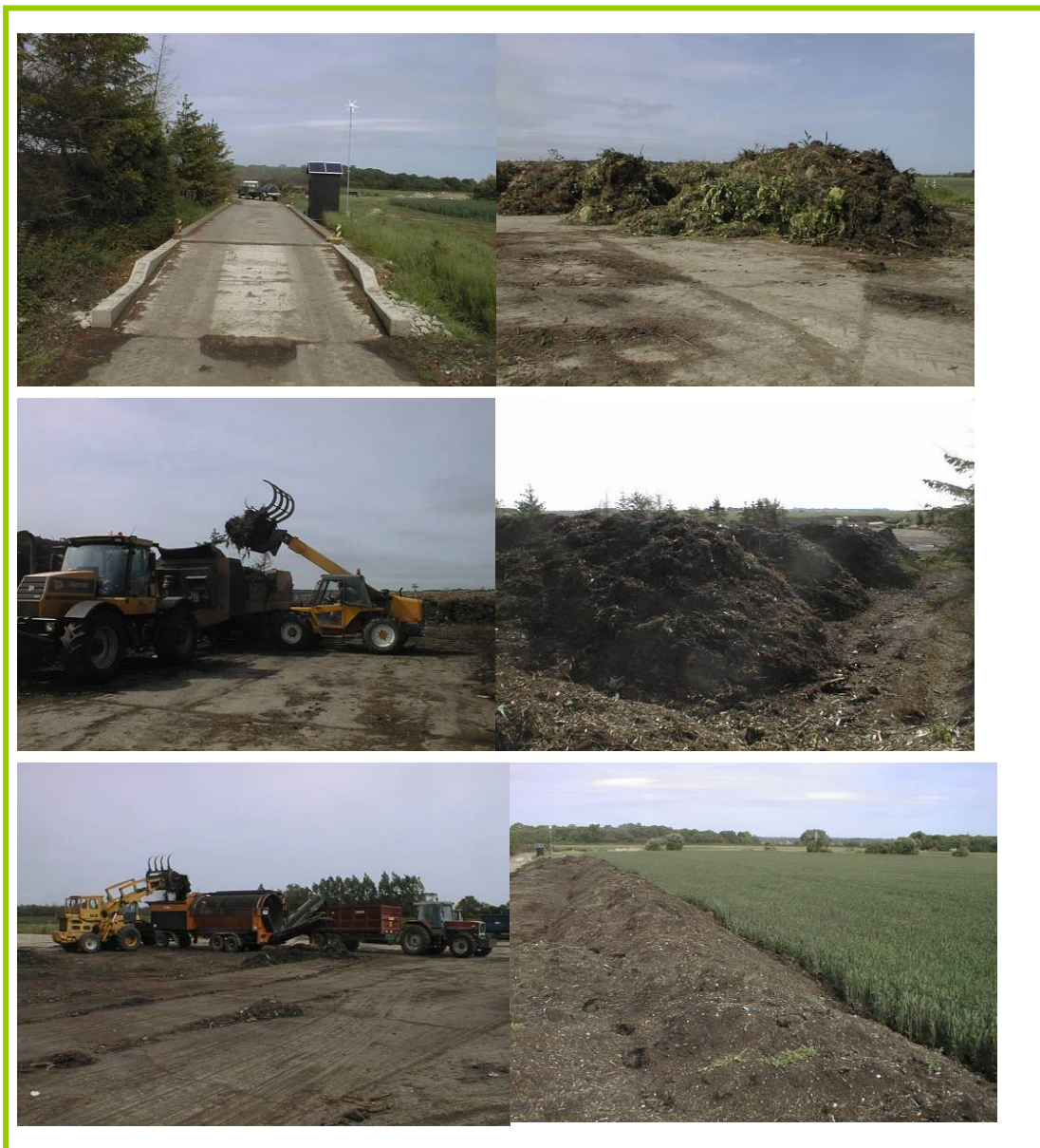
Figure 5 Colchester composting site showing weighbridge, green waste, shredding, windrows, screening and product stockpile awaiting harvest for application.
